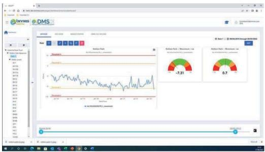
Figure 3: Screen shot from the iDMS portal of Rotton Park with Myview set up to indicate max and min levels of movement at a specific Hexagon.
