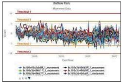
Figure 7: Movement across the whole dam. Showing an overall (small) down trend from 2019-2021 but a subsequent increase back to previous levels in 2022.
