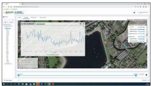
Figure 2: Screen shot from the iDMS portal of Rotton Park with three years' retrospective data – showing movement data graph associated with one hexagon.
