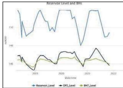
Figure 5: Water level and piezometer information at Rotton Park.
